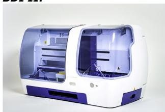
The BlueScan and Dr Dot Software are intended for reading test results of D-tek immunodot strips. The Dr Dot Software and BlueScan scanner have to be used in combination.
